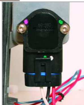
ETPAS dual redundancy pot for throttle lever
