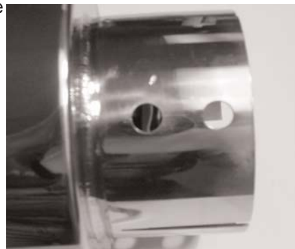
Holes in muffler attaching tube wall.
