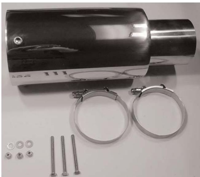
Each muffler is accompanied by two band clamps and three T-head 1/4-20 x 3" cap screws with nuts and washers. CAUTION: This muffler is intended to mount flush on the flat surface of the boat transom. This muffler weighs approximately 12 pounds.
