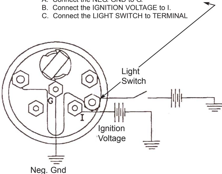
4. Reconnect battery ground. If meter does not read up scale, reverse meter leads.
