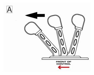
A) Forward cant models; arrow pointing to the ship's bow
