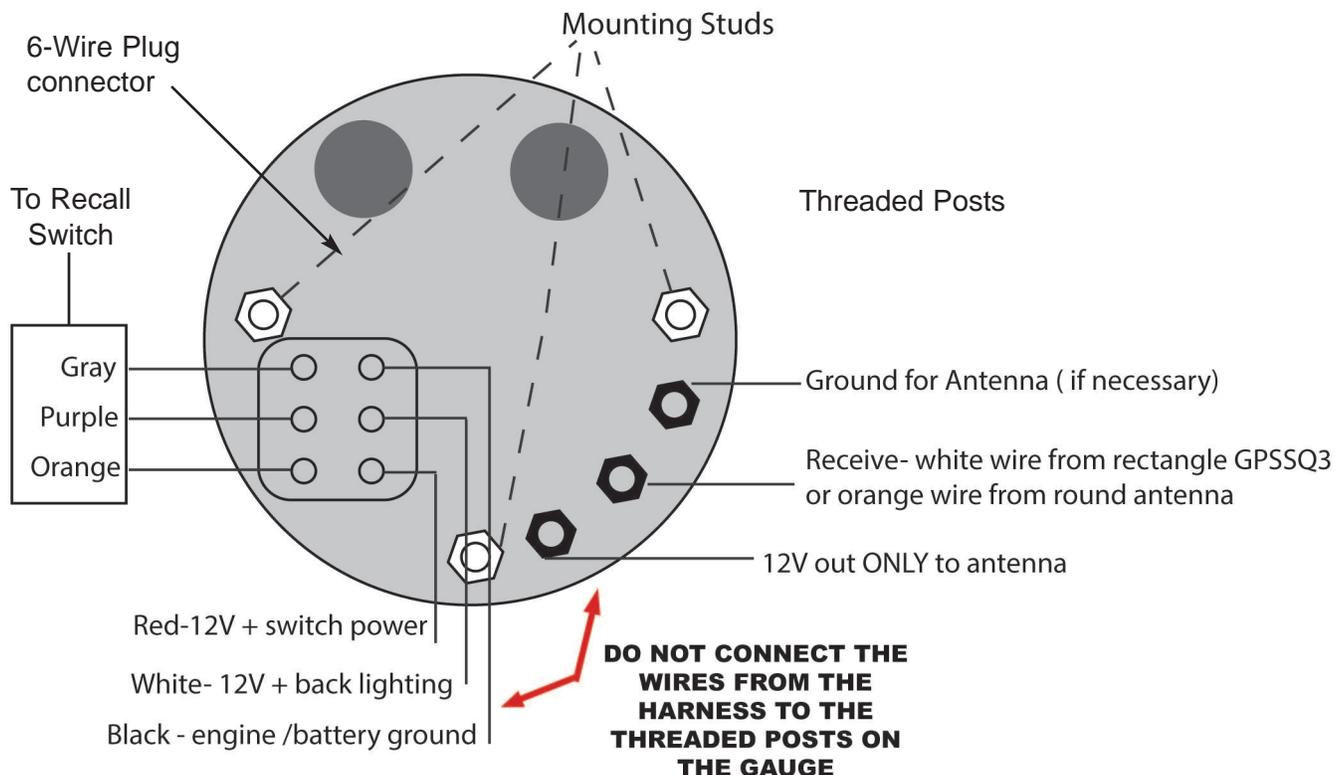
6. THE 6-WIRE PLUG WIRING TERMINATION
