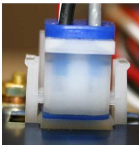
**STEP 4:** Push toward the other side so that the remaining locking tab clicks into a vertical position.
