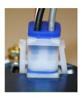
STEP 3: Push to one side of the plug, so that the locking tab clicks into a vertical position as shown here.
