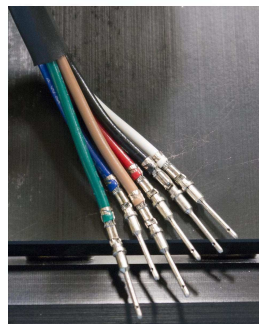
sensor wires from trim tab
