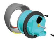
The visor Rim attaches by slipping the rim from the front of the gauge and slipping the bracket from behind, secure the bracket to the rim with screws and your done.
