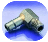
GCF7 5/16" x 24 thread male 90° angle to 1/4" push-on male
