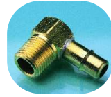
GCF6 1/8" NPT male 90° angle to 1/4" push-on male brass
