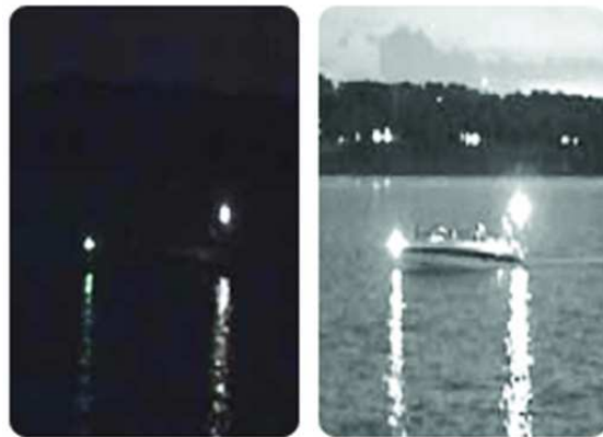
With a small amount of ambient light the low lux camera will give the operator a detailed picture unlike thermal.
