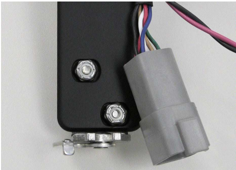
Neutral safety switch connection. Normally closed in neutral
